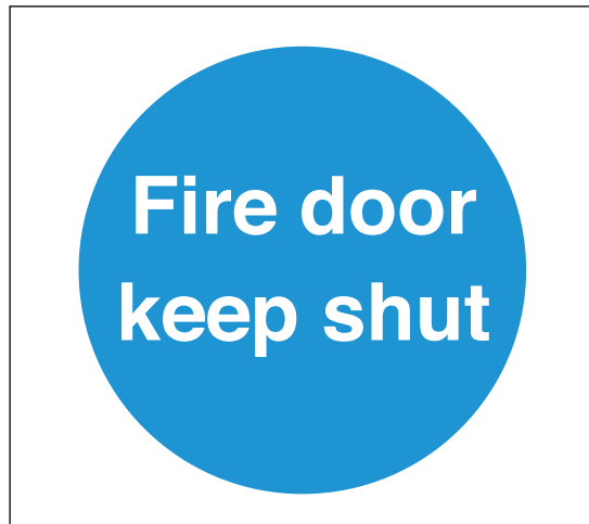
Figure 59: Fire door 'keep shut' notice
